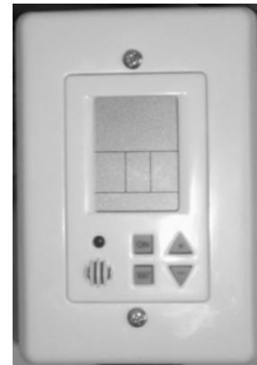
Figure 5 – Remote Thermostat Control
